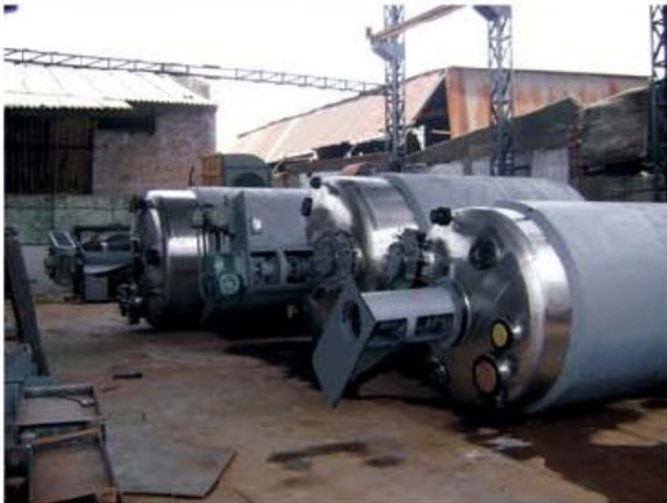
S.S. Jacketed Reaction Vessel With Mirror Finish
