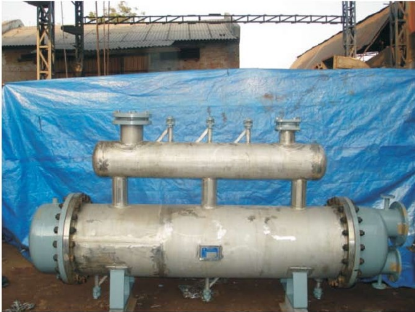
CO 2 Condensor With Expansion Shell For CO 2 Gas
