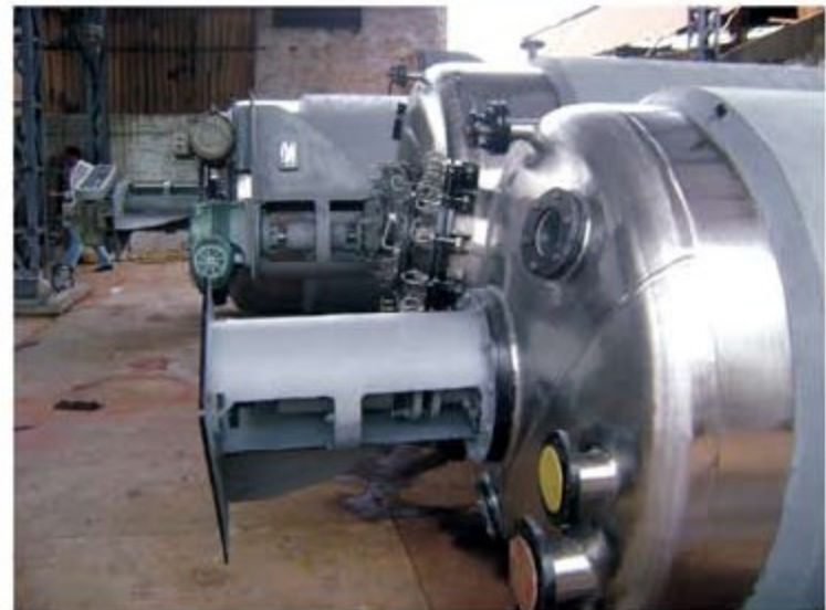
S.S. Jacketed Reaction Vessel With Mirror Finish
